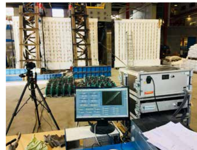
Experimental tests carried out at the Eucentre of Pavia (Italy) to verify the functioning of the ISOTEX construction system as a beam-wall.
