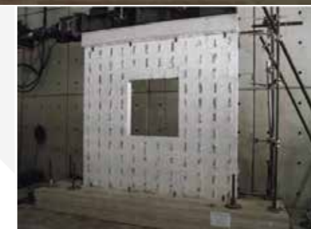
Left: Seismic test on ISOTEX two-storey wall Above: Seismic test on full ISOTEX wall Rights: Seismic test on ISOTEX wall with window
